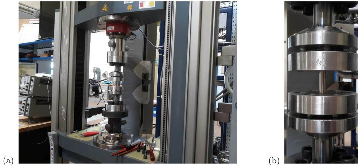
**Figure 7.1.:** (a) Experimental tensile test and (b) zoom into the holding device in which a cylindrical specimen is clamped.
