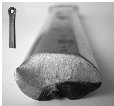
Figure 3.1: Failure by brittle damage of a bike's pedal arm. Image taken from Lokilech (2007).
