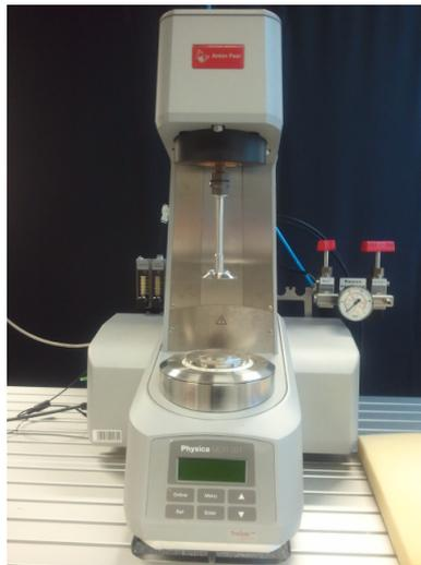
Figure 4.1: The Physica MCR 301 rheometer with plate-plate device
