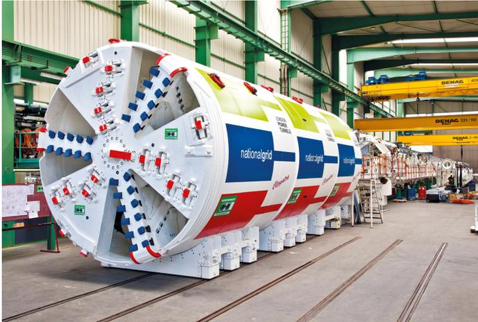
Figure 2.2: Earth Pressure Balance (EPB) shield TBM used in London. The diameter of the cutter head is 4.7 m. (Copyright: [www.herrenknecht.com](http://www.herrenknecht.com))
