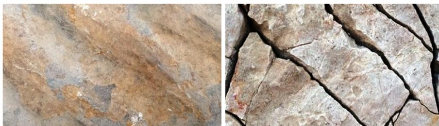
Figure 1.1: Example of an intact rock (left) and of a naturally fractured rock (right). Rock fractures often represent preferential flow paths that greatly increase permeability compared to fluid flow through intact rocks.
